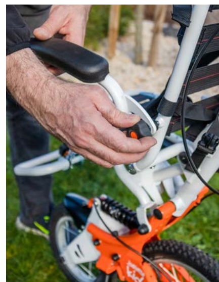
7. Pull up the armrests to screw them on the backrest with the rollers, while you adjust its inclination.
