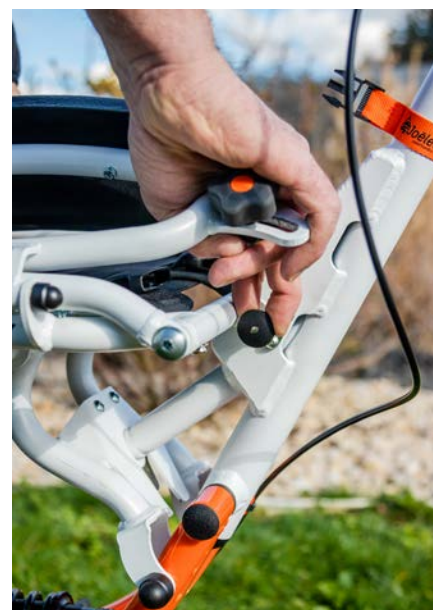
5. Tilt the seat in the print on the frame at the back with the indexing pin pulled.
