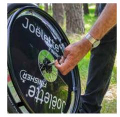
**9.** Insert the ball spindles until they lock (check that they lock by pulling on the wheel).
