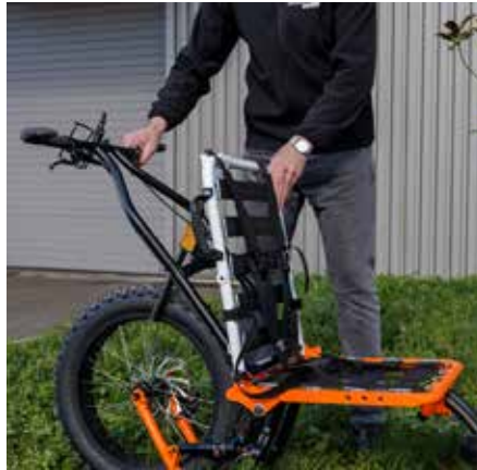
8. Unfold the backrest and lower the handlebars, using the handle on the left, to rest it on the wheel.
