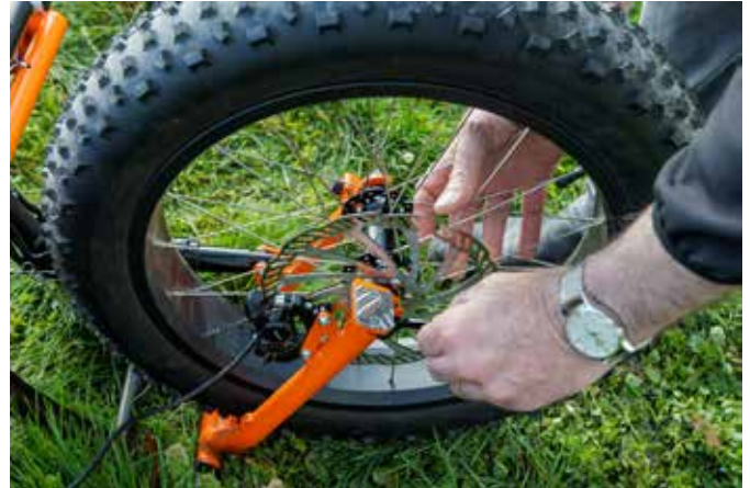
7. Position the wheel between the forks of the swingarm and secure it with the quick release.
