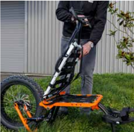
8. Unfold the backrest and lower the handlebars, using the handle on the left, to rest it on the wheel.
