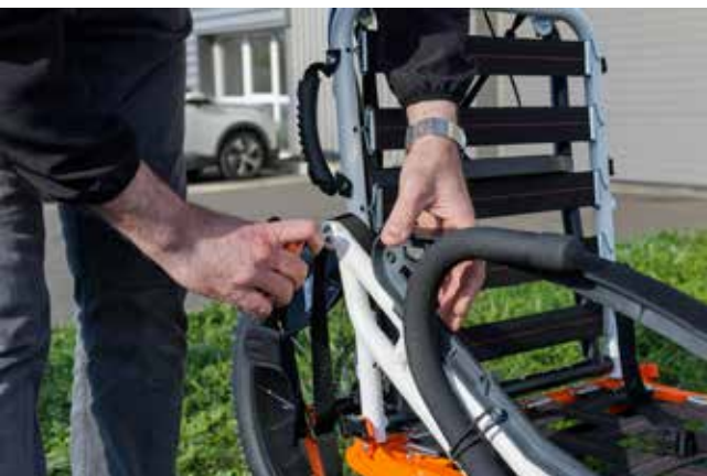
9. Install the two front arms with the side mounting screws.
