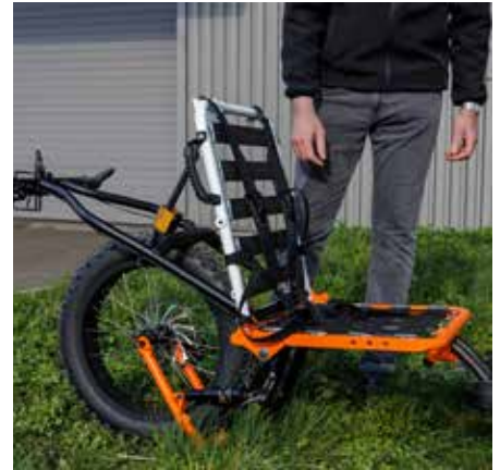
8. Unfold the backrest and lower the handlebars, using the handle on the left, to rest it on the wheel.
